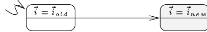
Figure 3: Automaton representing the set of input vectors for the two-vector delay model. \vec{i}_{old} and \vec{i}_{new} represent the vectors of primary inputs before and after time 0. \vec{i}_{old} and \vec{i}_{new} are selected non-deterministically, which enables the automaton to represent all input vector pairs.
