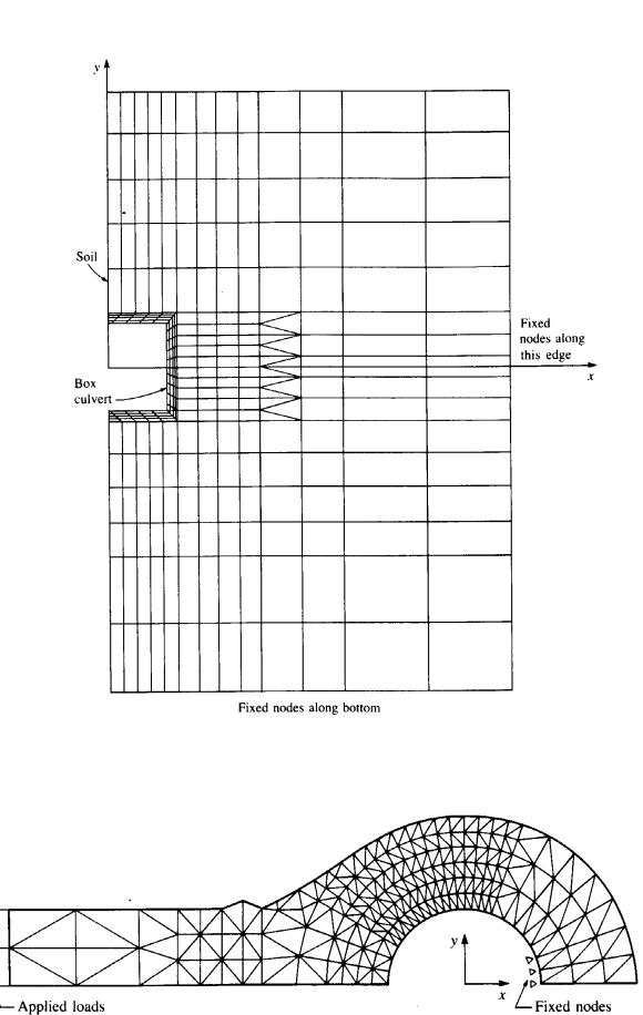
The *axisymmetric element* is developed by rotating a triangle or quadrilateral about a fixed axis located in the plane of the element through 360°. This element can be used when the geometry and loading of the problem are axisymmetric
