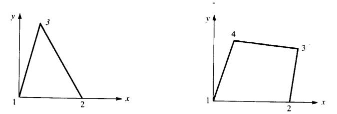
The simplest two-dimensional elements have corner nodes only (linear elements) with straight sides or boundaries although there are also higher-order elements, typically with mid-side nodes (called *quadratic elements*) and curved sides. The elements can have variable thicknesses throughout or be constant. They are often used to model a wide range of engineering problems.
