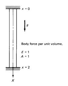
4. Use Galerkin's method to find the displacement of the midpoint of the rod in Problem 3.
