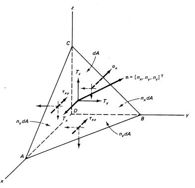
where **DA**, **DB**, and **DC** are parallel to the *x*, *y*, and *z* axes, respectively, and the area **ABC**, denoted by **dA**, lies on the surface. If the unit vector normal to the surface **dA** is given as:
