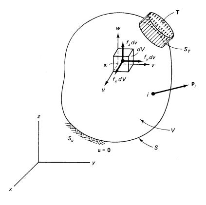
A point in the body is located by *x*, *y*, and *z* coordinates. On part of the boundary, a distributed force per unit area *T*, also called *traction* is applied. Un-
