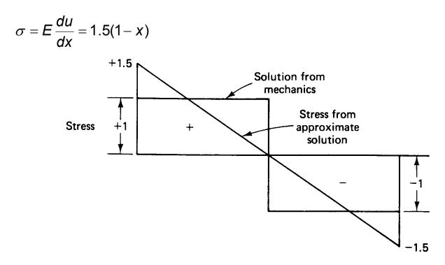
Notice that an exact solution is obtained if a piecewise polynomial interpolation is used in the construction of u.
