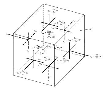
When the volume dV shrinks to a point, the stresses may be represented by placing its components in a (3 x 3) symmetric matrix. Stress can be represented by the six independent components:
