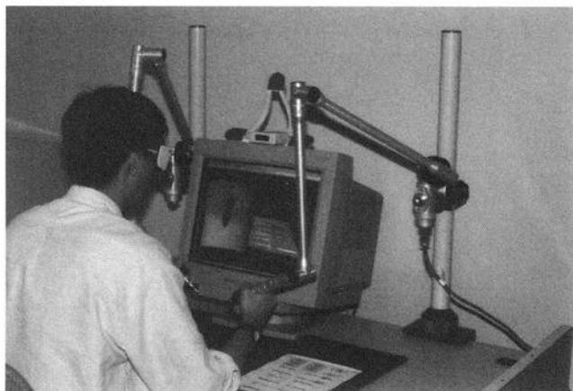
Figure 3. Photograph of surgical simulation system. The user views the virtual thigh model through stereo glasses synchronized to the computer screen. He manipulates the virtual surgical instruments using six degree-of-freedom input devices. Switches on the devices are used to select a particular instrument, and to perform instrument-specific functions, such as gripping and releasing objects with the forceps.
