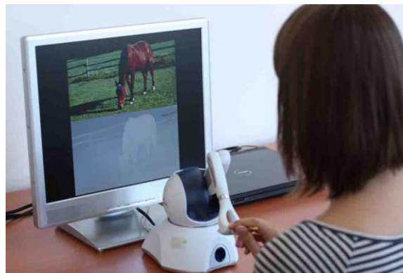
Figure 6. The demo set-up with a 2D video display and a haptic cursor. The pixel touched is indicated by the cursor, which helps user navigate and experience the haptic scene and haptic motion.
